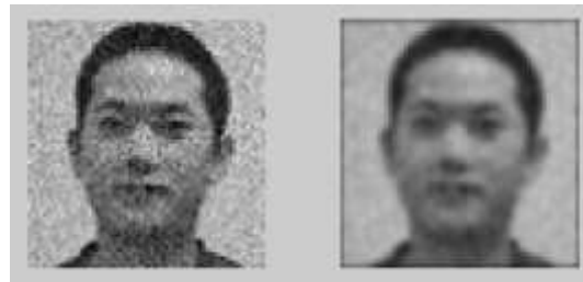
Figure 5 (a) Degraded Image (b) Gaussian filtered Image
